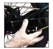
These two pictures show the correct tension. When pushing up on the chain, it should only move between 5 and 10mm.
