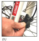
**7.** Loosen top calliper Allen bolts (*picture 3 - using 5mm key*) - so it will move side to side so as to aid fitting of wheel.
