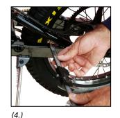
**6.** To re-install the wheel reverse the above procedures. Ensure the chain is correctly adjusted and lubricated, the wheel is aligned, and all nuts and bolts are tight *(image 4).*
