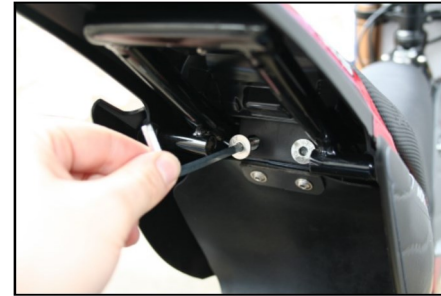
(1.) Unscrew & remove seat bolts.
