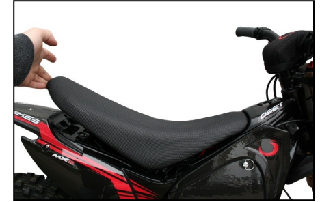
(2.) Lift seat up & forwards to release.
