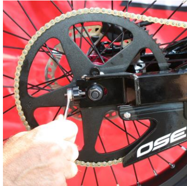
Chain tensioner nut (13mm).
