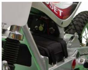
The 'switch-plate' is located beneath the seat area, behind and above the batteries. As the rider sits, the key switch is on the right, the back side of the 'speed dial' potentiometer is in the middle, and the charge port on the left. Please note, the toggle switch in this picture has been replaced by a key switch on production models.
