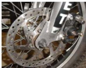
The Spider 16.0 features a front disc brake, as opposed to the 'V' Brake on the Spider 12.5.
