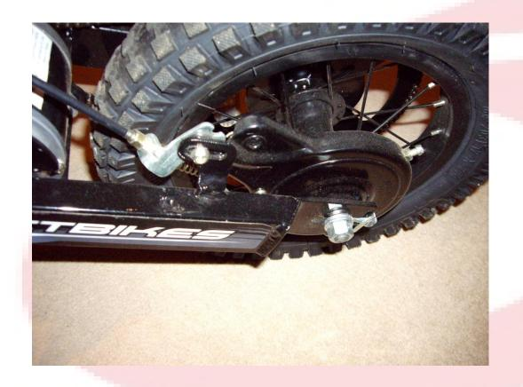
2.3 (cont) – The Rear Band brake is mounted on the swing arm. There is a small amount of adjustment at the end of the cable here, check that the band itself is not dragging on the braking surface, ensure that the internals on the band brake are not damaged and that the brake is free from debris.
