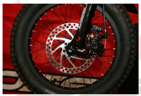
2.3 – Cable operated mechanical disc brakes - cable tension adjustment can be made via the barrel adjustment on the lever and at the calliper. Lever reach adjustment can be seen above by using a 2.5mm Allen key. Again always ensure that before you make any adjustment the wheel is sitting square in the fork dropouts and that the quick release system is firmly secured. Spin the wheel to check the disc is running true.
