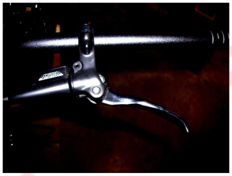
2.3 – A Hydraulic Brake upgrade is available for all 16.0 models. The Tektro Auriga Comp has been modified by OSET so that hose lengths are a correct fit. While the brakes do come with full instructions, we have included the basics here.
