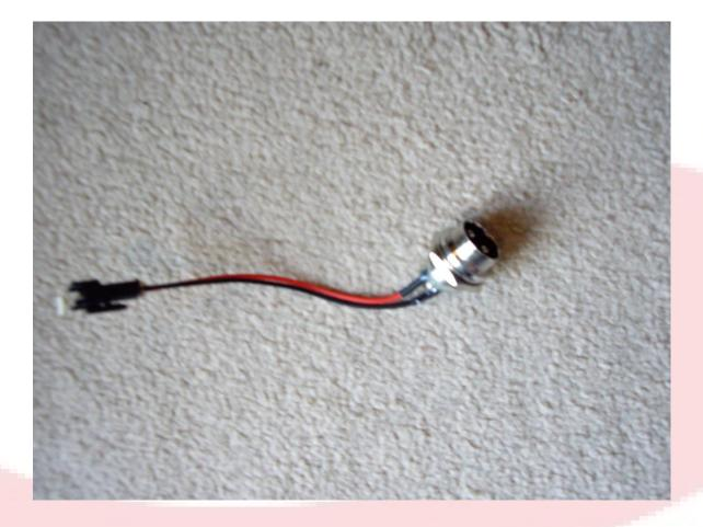
3.5 - Here you see a charge port removed from the OSET. The charge port connects into the wiring harness. Ensure that the wires look in good shape and that the back of the port is still well sealed with resin. It is a very simple component and as a result there is little that could go wrong.
