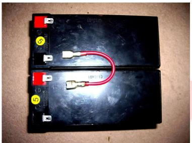
2.1 – The Voltage output of the batteries can be checked by means of a Multimeter. Measure each battery individually by placing the electrodes of the Multimeter across the terminals.
