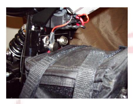
1.1 – The potentiometer on your OSET is located between the key switch and charge port just above the battery tray. The potentiometer can be adjusted from the rear with a flat blade screwdriver through the access hole in the rear splash guard.
