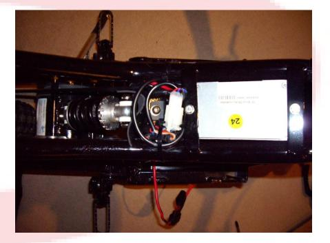
1.3 – The Relay pictured to the left 'off the bike' and above located on a 12.5 24v. To remove simply undo the 4mm Allen bolt securing it to the frame, disconnect the key switch at the black connector and from the wiring harness via the larger white connector.
