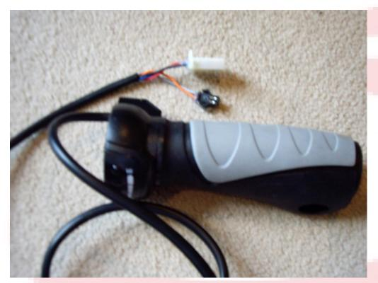
5.1 – Here the throttle is removed from the OSET. In 99.9% of cases faults with throttle will be a direct result of the bike being dropped on its right hand side. While there may be no visible damage, the resistor in the throttle body could have been damaged, resulting in either an intermittent message to the controller or no message at all.
