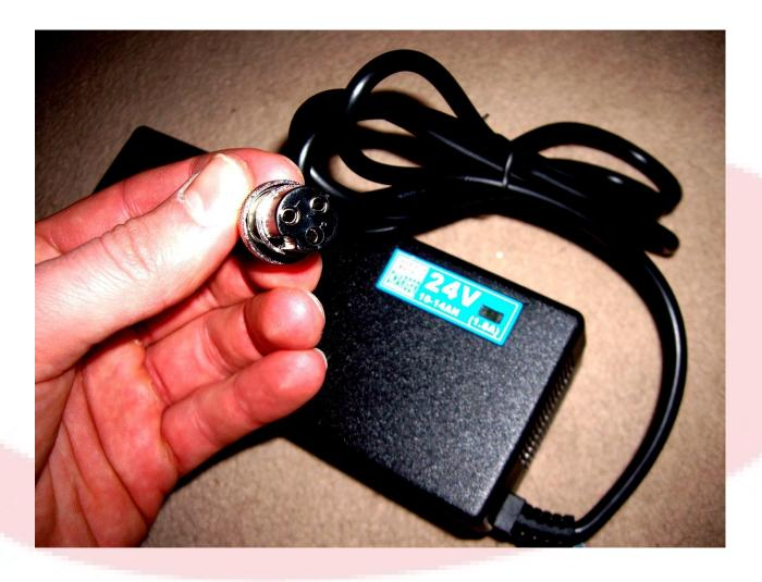
3.2 – Place the electrodes from your multimeter into the top two holes on the charger to bike lead to get your voltage output reading.
