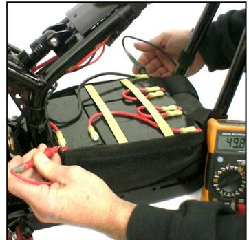
If different batteries show different readings then the ideal course of action would be to 'balance' the batteries (*see below*). The multimeter is also very useful in diagnosing any electrical problems on the bike.
